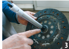
Insert the centering tool into the disc.
