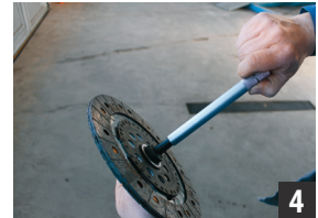
Fasten the tensioning screw so that the tool completely fits the disc.
