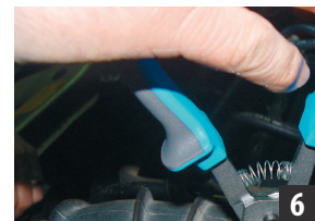
When the special click is heard, the clamp is correctly fastened.
